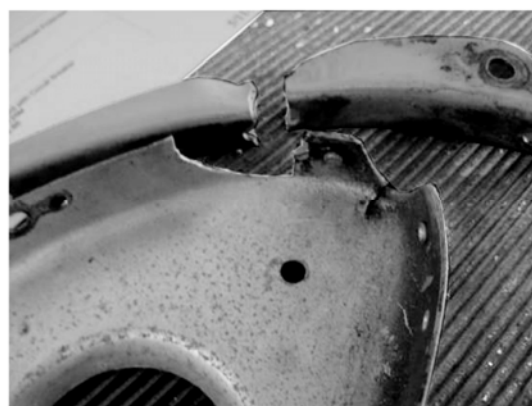
EXAMPLE OF TORN FLANGE IN P/N 35-165050-84 WITH NUTPLATE MISSING
