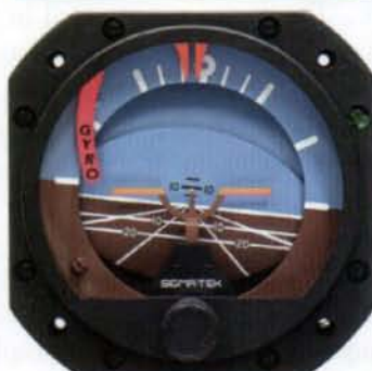
These artificial horizons can provide you with prompt notification (red flags) of a failure of the instrument or vacuum source.
