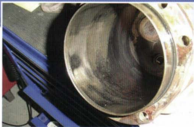
Badly corroded IO-520 cylinder (all six were damaged) from an engine with the heater left on all the time. This airplane is flown very regularly so a lack of oil coating due to inactivity is not an issue. See text for details.
