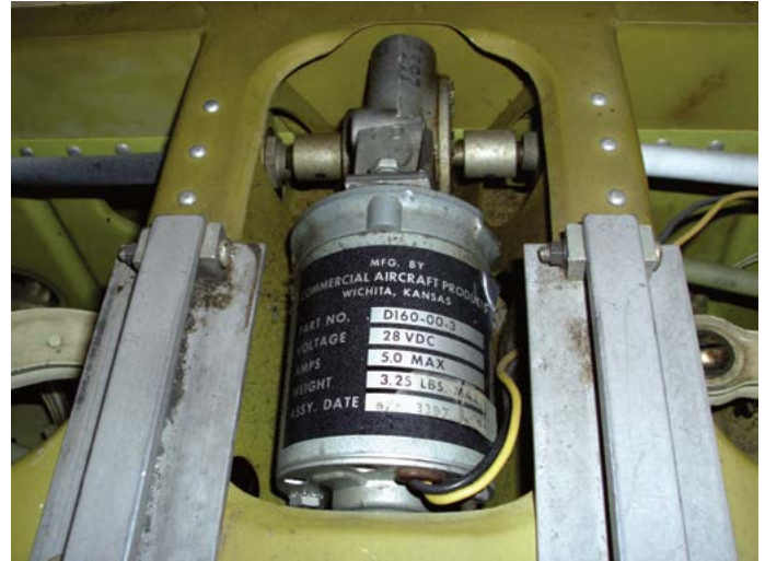
Flap motor (B55 installation shown; similar in D35).
