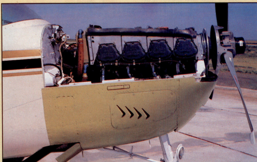
Installation of the 568-pound IO-720 does not alter the CG limits of the A-36 Bonanza.
